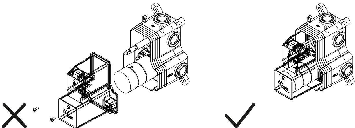
EN CASO DE SOLDADURA-IN CASE OF WELD-EN CAS D'INSTALLATION PAR SOUDAGE
